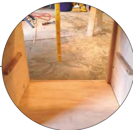
STEP 13. The next job is to measure the centre shelves and secure with pocket screws
